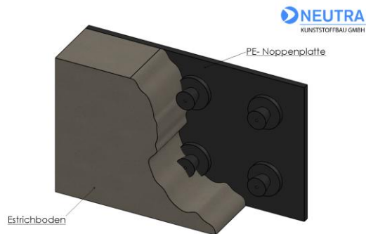
Fig. 2: Neutra flooring layers: Screed/ Knobbed PE tile
