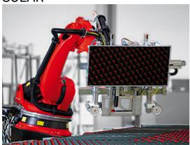
The Grenzebach solar module production lines are the embodiment of our decades of experience in glass processing and finishing. For our international customers we are planning and realizing crystalline and thin-film photovoltaic lines, production lines for the concentrator technology (CPV and CSP) and assembly and module lines - including customized feeding and assembly technology, robot and inspection system and accumulators.
