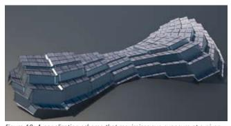
Figure 10: A panelization scheme that maximizes sun exposure at a given time
