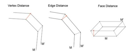
Figure 3: The three different ways of measure the distance between meshes
