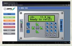
Dial up via a password protected IP-address and have a 1:1-view of the weighing calculator with full functionality in your browser window.
