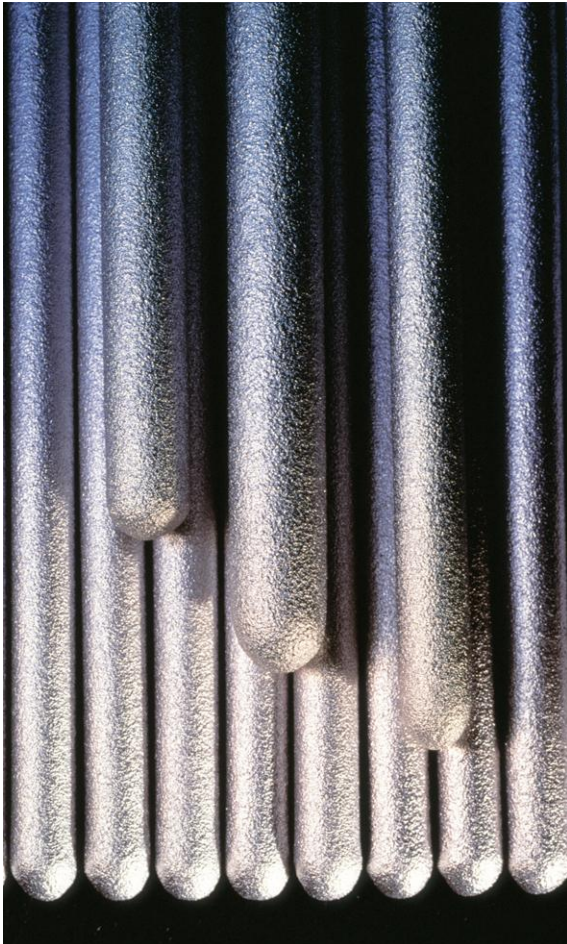
Thermocouple sheath of different diameter, ACT ® coated with a platinum/rhodium alloy
