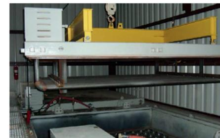
*An overhead crane is used to remove the top lids from the catalytic filter's modules to provide easy access to the collection filters.*
