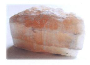
Soda ash can be made synthetically using limestone, salt and ammonia. This is known as the Solvay process, and was the main source of soda ash until deposits were discovered. However, it is more expensive than mining natural sodium carbonate deposits. In addition, the waste products of this process are harmful to the environment and could cause serious waste management problems.
