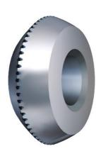
Due to its patented wheel structure with small notches, the Penett® wheel creates a very deep median crack of up to 90% of the glass thickness, which effectively simplifies or even eliminates the breaking process.
