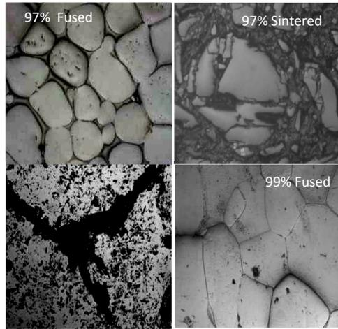
**Figure 1:** Microstructure of different Magnesites
