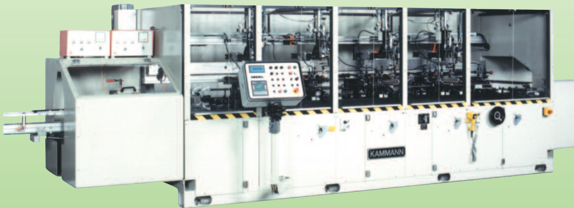
project drawing of a 4 color K 14-U with transfer stations for upright article in- and outfeed and integrated UV curing aggregates
