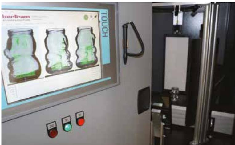
Separator with the door open, showing the user interface and a jar passing through the camera system.
