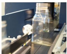
Allocators are integral parts of inline-sorting, above all, in bottling plants and the food and drink industry. Due to the high production speed, modern systems work with powerful control systems, highly dynamic drive technology and precise industrial image processing. We have developed our own Allocator based on our comprehensive know-how of the container glass manufacturing process. This combines image processing, SPS and servo-motor drive technology into a compact and easy to integrate unit.
