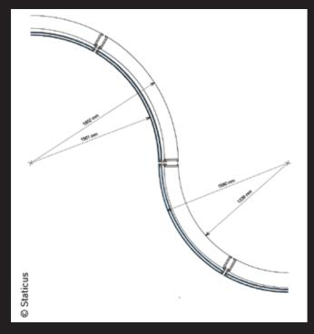
The curved insulating glasses in the facade of Våghuset have radii of 1580 mm for the convex and 1561 mm for the concave elements
