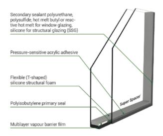
Fig. 1: Flexible spacer Super Spacer® with integrated desiccant, vapour barrier and lateral acrylic adhesive.
