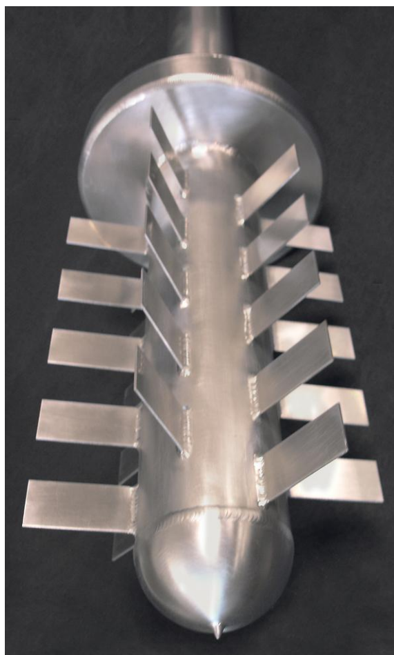
Fabricated stirrer, made of rhodium/platinum sheet, design from Füller Glastechnologie
