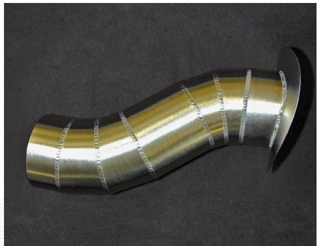
Fabricated tube made of platinum/rhodium sheet
