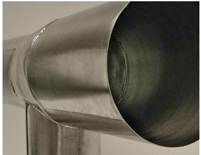
Fabricated chamber made of iridium sheet
