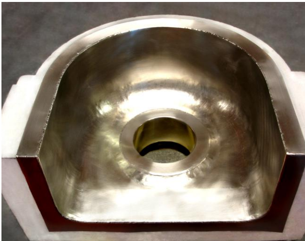
Spout bowl, protected with a lining made of ZGS platinum/rhodium sheet
