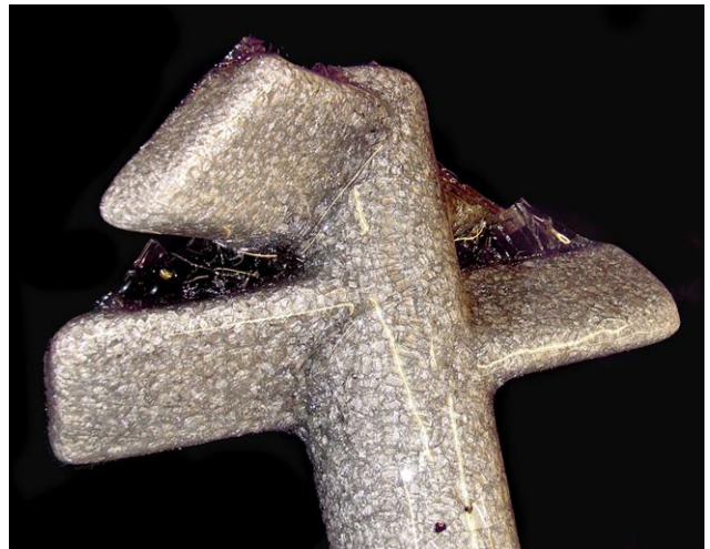
Ceramic stirrer returned for refining, fully protected by ACT ® during a two-year campaign
