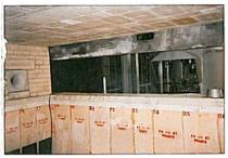
will, FIC has adapted its comprehensive in-depth forehearth sealing technology to create a unique, sealed, electric furnace with hot-top which allows a flexibility of operation never before available in an electric furnace. Idling a traditional cold-top electric furnace will cause blanket melt-out.
